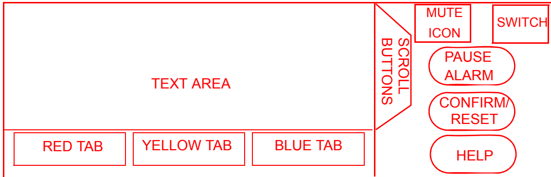
Figure 1-8. Alarm/Information Messages Area
